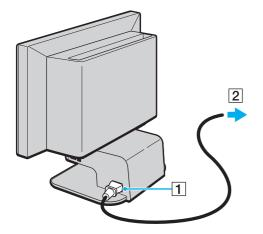
To disconnect the computer completely from AC power, unplug the power cord.
